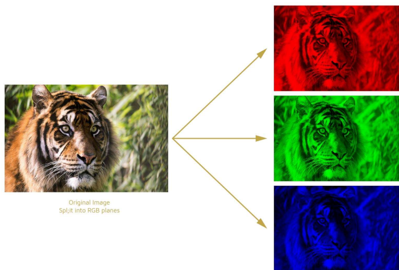
Figure 6 - An image decomposed into RGB planes
